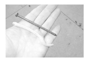
2 Using a nail or drill, make a hole in the lid, roughly centered, that will be just large enough for the wick to slide through. You're going to want the wick to be snug, so don't make the hole too big. Also, make a small hole in one corner of the lid. This allows air to get into the tin.
