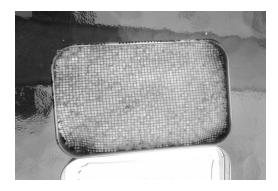
4 Carefully pour the alcohol directly onto the screen. You don't need a lot; just 3 tablespoons will suffice in most cases. After closing your fuel bottle and placing it well away from the tin, light a match and place it directly onto the screen. The alcohol fumes should light instantly. Be advised, alcohol burns very hot and the flame can be difficult to see. If you aren't sure whether the stove lit or not, slowly move your palm near the stove to feel for heat.
