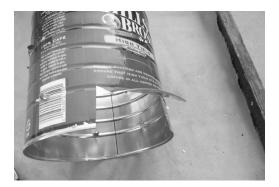
4 You can see here where I crimped over the jagged edge left from the long cut. This is done by cutting approximately ¼ inch deeper on each side of the door. Start at one end of this thin flap and bend the metal over to the inside of the can.
