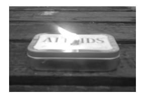
**6** When storing this expedient lamp, be sure to empty the oil from it first. Because of the holes in the lid, it would be far too easy to accidentally spill oil if it is knocked around.
