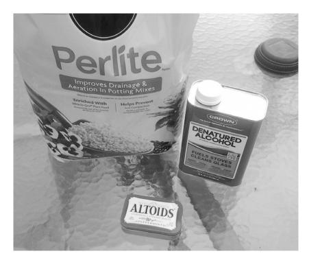
\* Perlite and vermiculite can both be found in most garden stores. It is a relatively inert soil additive that looks like small white rocks. This substance soaks up the fuel and releases it slowly, just as it would with water in a garden. Look for products that don't have chemicals, such as plant food, added. If you can't find
