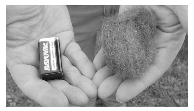
1 For this project, all you do is connect the positive and negative battery terminals with a piece of steel wool. The wool will quickly begin to heat, glow, and flame up.
