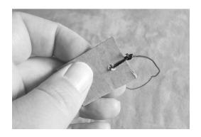
**6** Position the alarm in such a way that the clothespin is attached to something fairly stationary, such as a wall or a heavy piece of furniture. The trip wire runs from the interruptor to another fixed point, like a nail or screw attached to the wall at the opposite side of the hallway. If both the clothespin and the other end of the trip wire are both firmly anchored, the trip wire will pull the interruptor from the clothespin when the wire is tripped.
