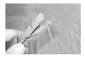
**3** Next, take a new wire and remove the insulation from the end, then wrap it around the other jaw of the clothespin.
